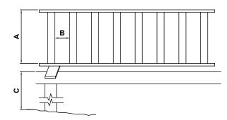
MATERIALS USED IN AREA A MUST NOT FACILITATE CLIMBING (ie: LATTICE, HORIZONTAL MEMBERS, ETC.) SECTION 9.8.8.5 N.B.C.
